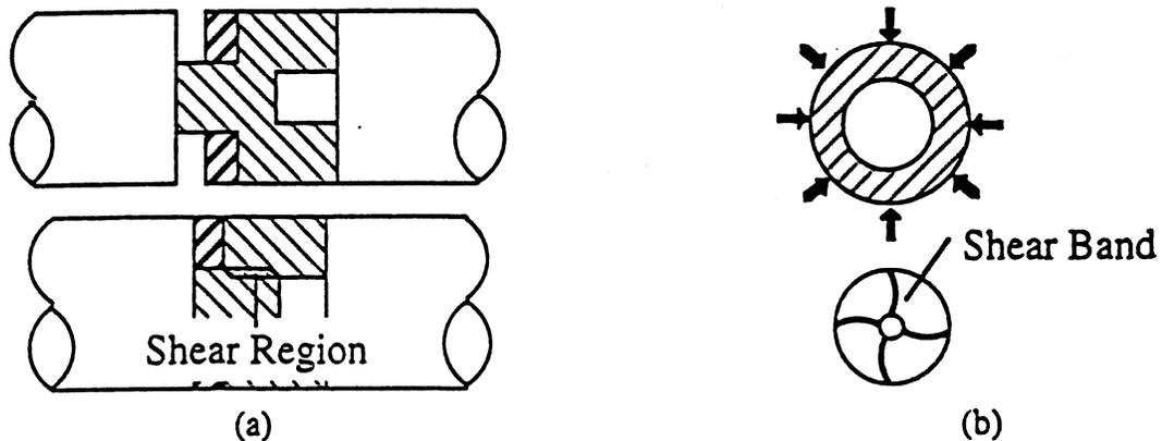
Figure 2 Two experimental techniques applied for large strain, high strain-rate deformation of metals: (a) hat-shaped specimen; and (b) thick-walled cylinder method.
