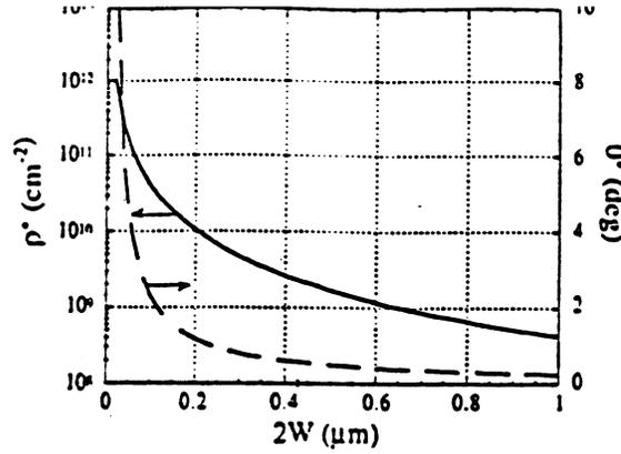
Figure 7 Critical dislocation density  $\rho^*$  and resulting misorientation angle  $\theta^*$  as a function of cell width  $2W$ .
