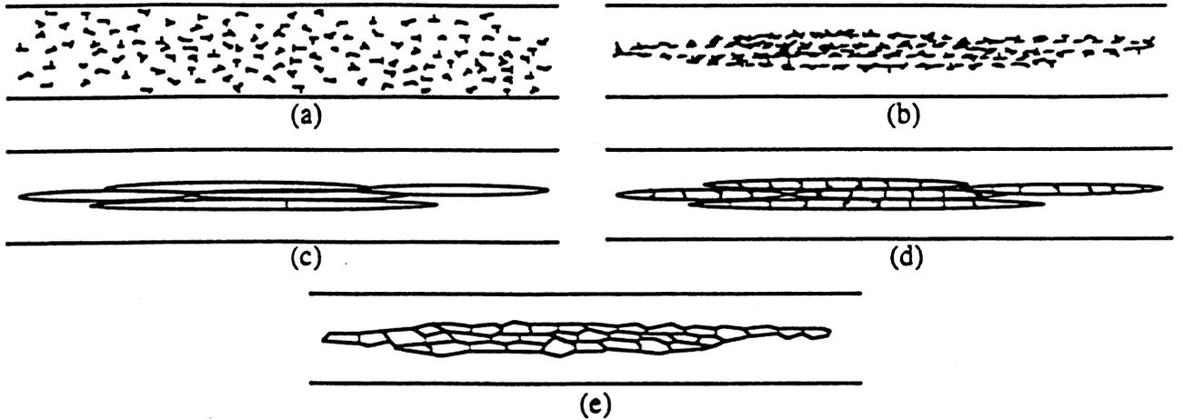
Figure 6 Schematic illustration of microstructural evolution during high-strain-rate deformation. (a) Randomly distributed dislocations; (b) Elongated dislocation cell formation (i.e. dynamic recovery); (c) Elongated subgrain formation; (d) Initial break-up of elongated subgrains; and (e) Recrystallized microstructure.
