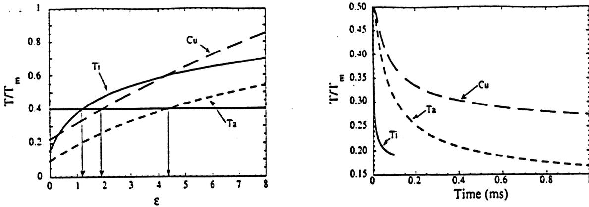
Figure 5 (a) Normalized temperatures as a function of plastic strain for titanium, copper, and tantalum. (b) Shear-band cooling curves for titanium, copper, and tantalum.
