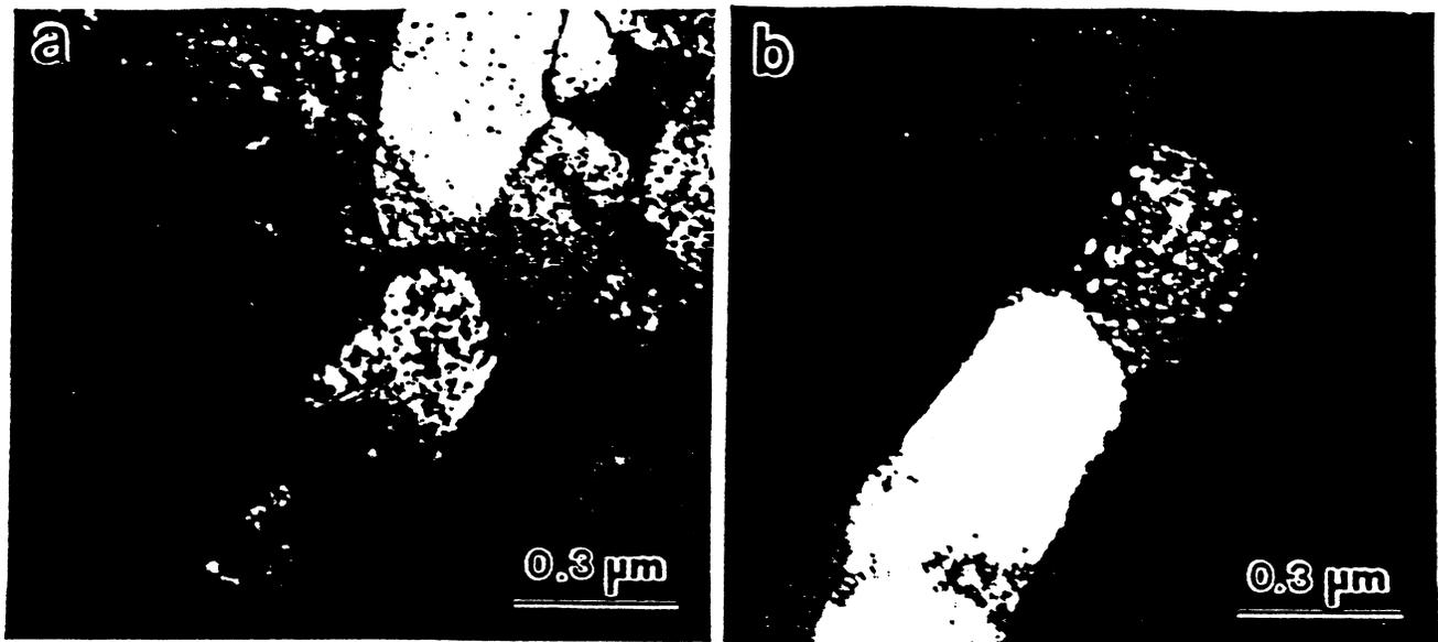
Figure 4 TEM micrographs of microcrystalline structure generated in tantalum. (a) bright field; (b) dark field. (From Nesterenko et al. [14]).
